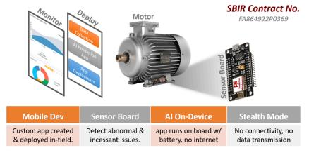
Mobile devices are connected to a sensor-board on motor/equipment with USB or BLE protocol to receive sensor data, train/test AI models, compile and deploy firmware to monitor health. Our solution provides high to machinery equipment operating in austere environments since it runs on battery and requires no Internet connection. By accurately predicting the
